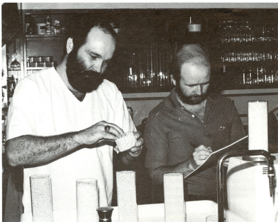
Mr. David Rutland (left), IFDC Chemical Laboratory Analyst, and Mr. David B. Wright, IFDC Technical Aide, conduct hygroscopicity tests on rubber-coated urea.
