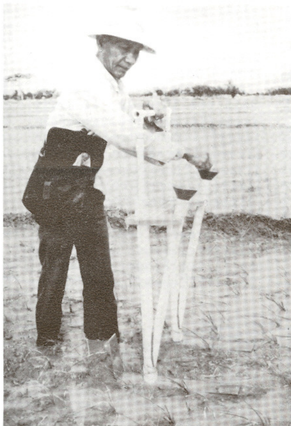
A Philippine farmer uses the urea-briquette applicator.
