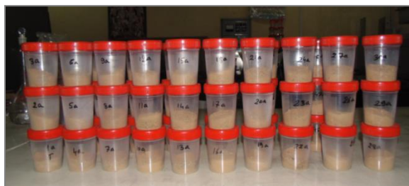
Figure 52. Soil incubation experiment to study the P release from different CPCs loaded with oxalic acid and PSB
