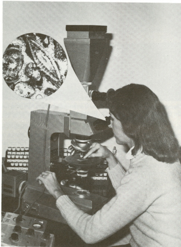
Using a polarized-light microscope, Ms. Michelle Cooper, Mineralogist, examines a petrographic thin section of Leyte phosphate rock.
