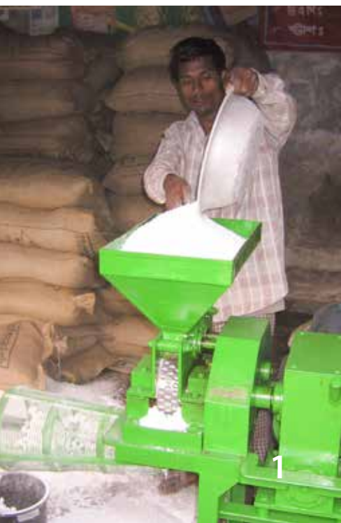
▲ 1) Prilled urea is poured into a briquetter. 2) A briquetter produces briquettes. 3) FDP briquettes. 4) The relative size of briquettes is shown.
