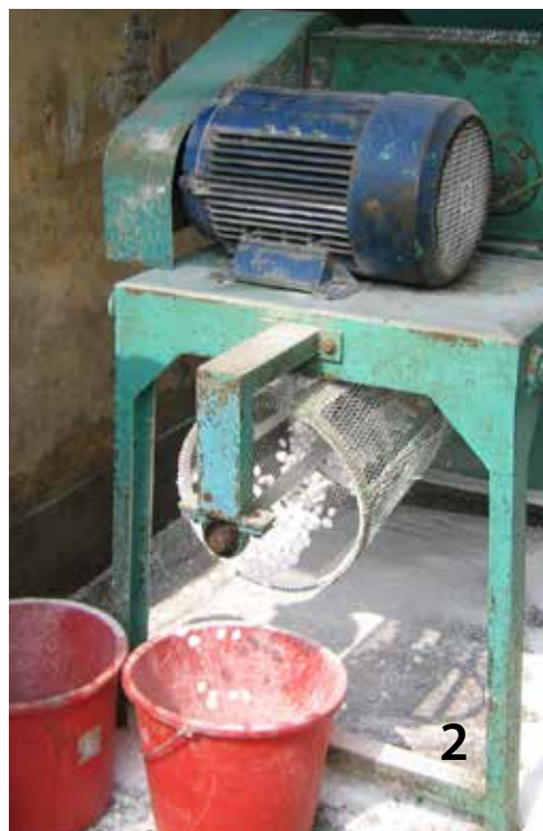
▲ 1) Prilled urea is poured into a briquetter. 2) A briquetter produces briquettes. 3) FDP briquettes. 4) The relative size of briquettes is shown.
