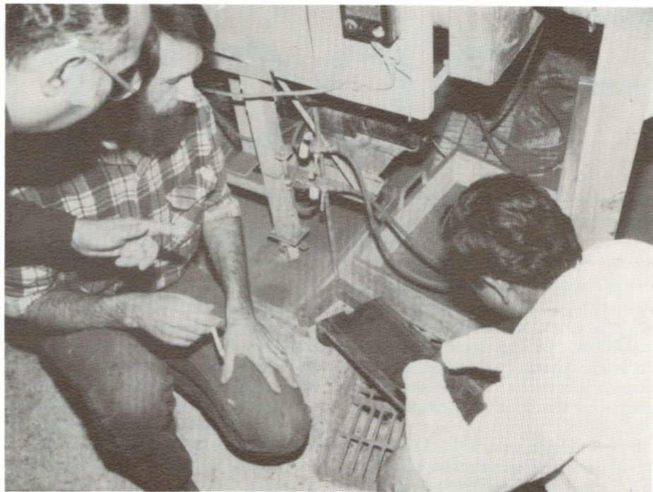
R. K. Puri, PPCL Mechanical Engineer (left); IFDC Technical Aide M. E. Goode; and B.V.M. Rao, PPCL Project Coordinator, examine the shell of a pinmixer, which was used in the minigranulation trials.
