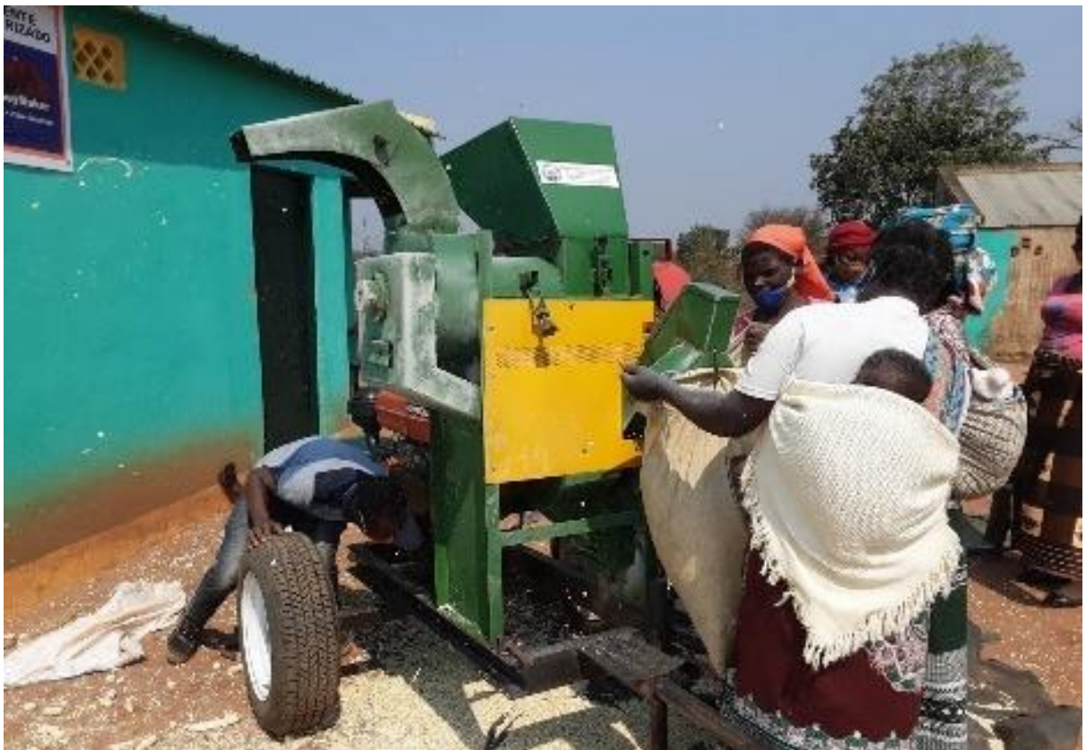
Use of maize thresher to reduce labor for women and improve grain conservation with a view to reducing post-harvest losses
