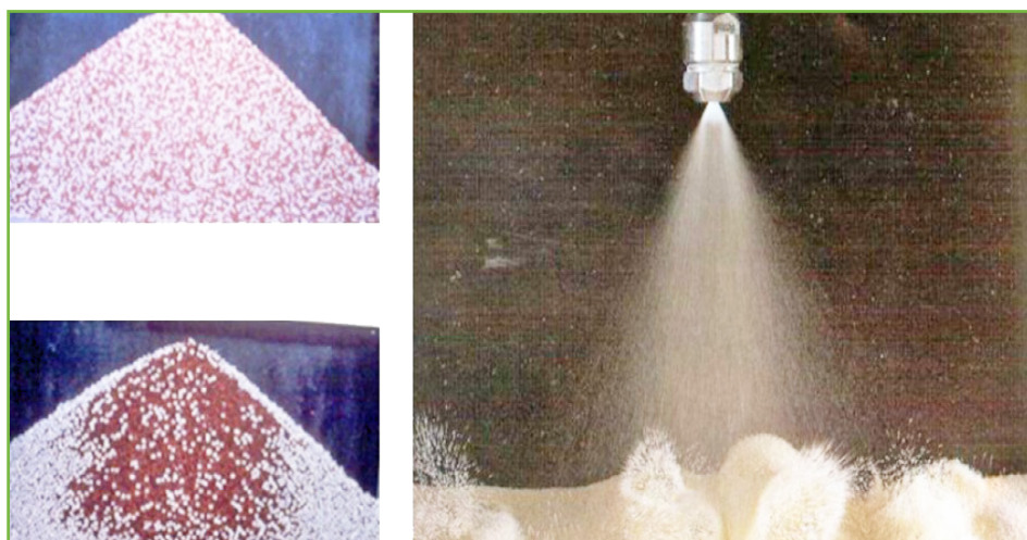
FIGURE 7. Mixing fertilizers with risk of segregation (left) and incorporating trace elements into granulated fertilizers by coating (right)
