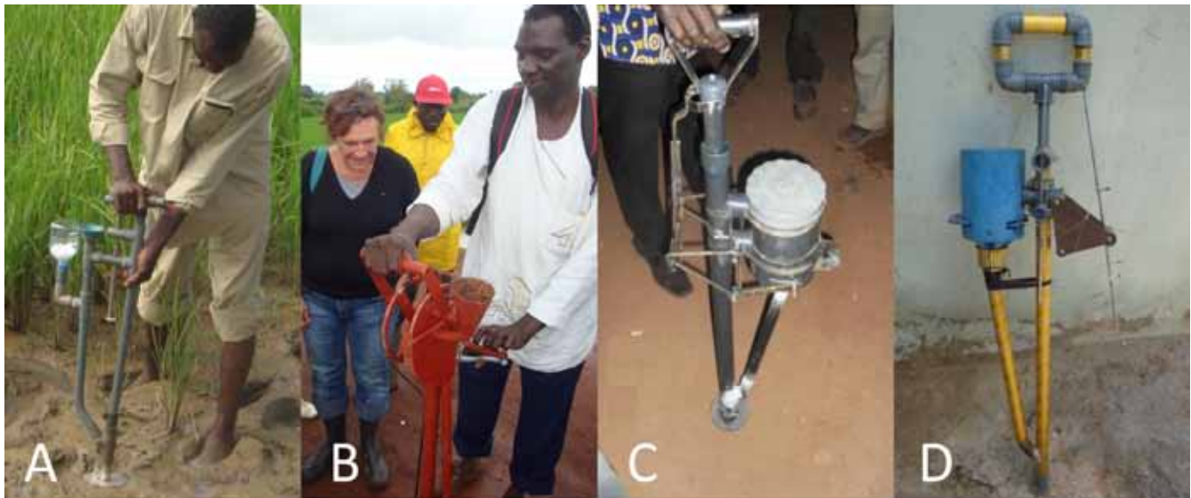
▲ Different types of FDP applicators were studied, designed and tested in 2010 and 2011: (A) Bangladeshi injector-applicator; (B) applicator prototype developed by a local blacksmith; and (C and D) local applicators developed by MATAGRI Conceptors.
