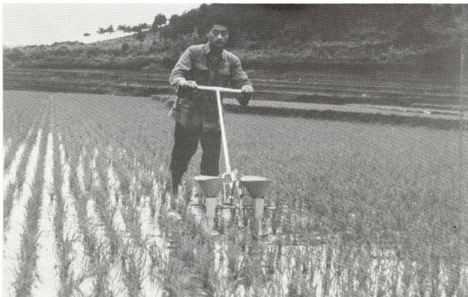
An FAAS staff member demonstrates the use of a deep-placement applicator for urea supergranules on paddy rice.
