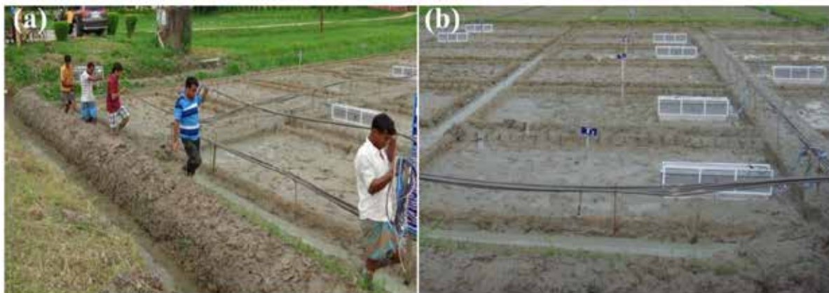
Figure 4. Installation of Gas Chambers (a) Carrying a Chamber into the Field and (b) Installed Chambers in Field
