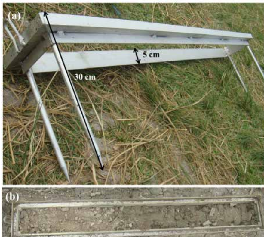
Figure 2. Chamber Base Frame (a) Before Installing in the Field and (b) After Installed in the Field
