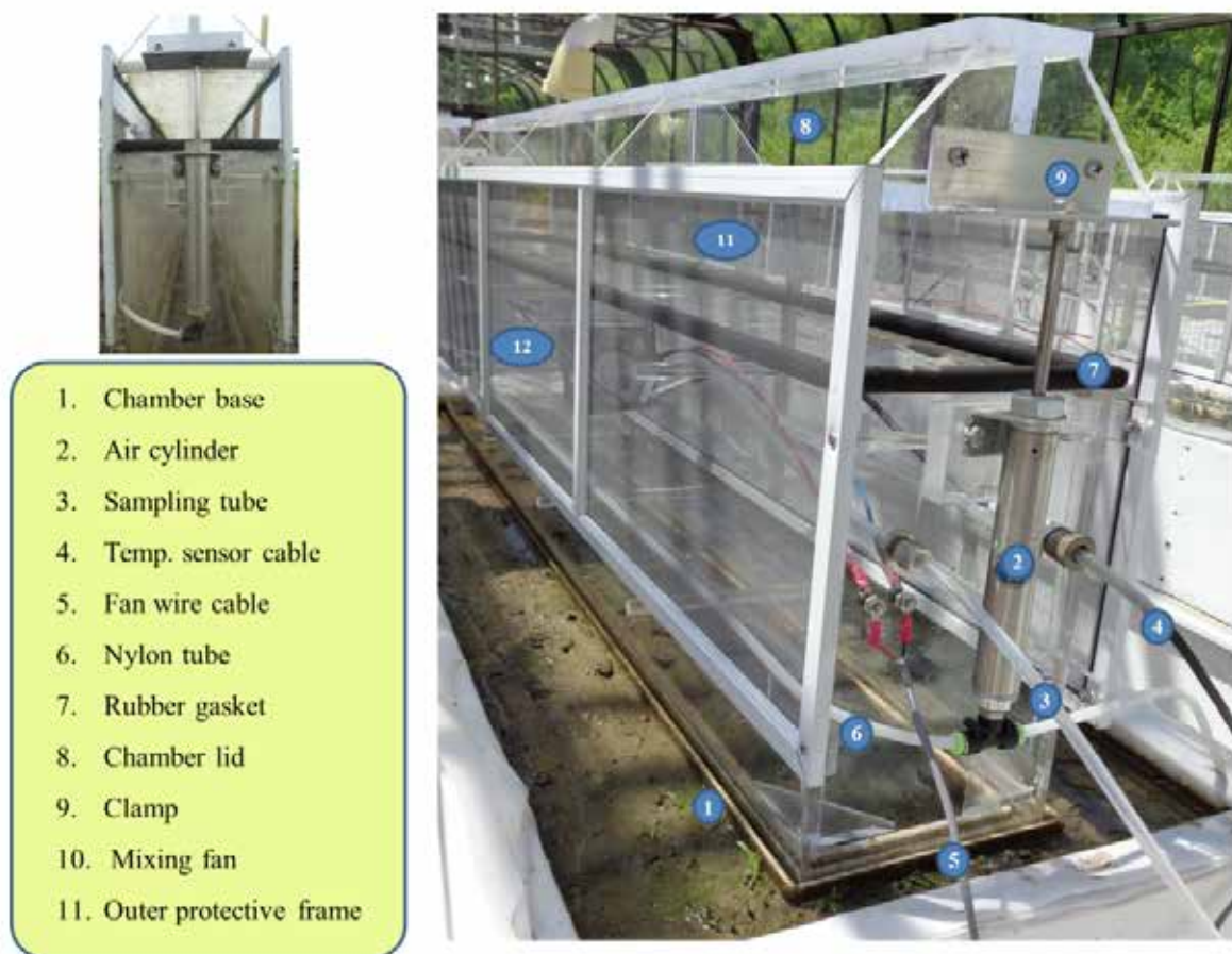
Figure 1. Gas Chamber (in an Open Position) Showing Different Parts; Inset Picture Shows the Breadth Side of the Chamber
