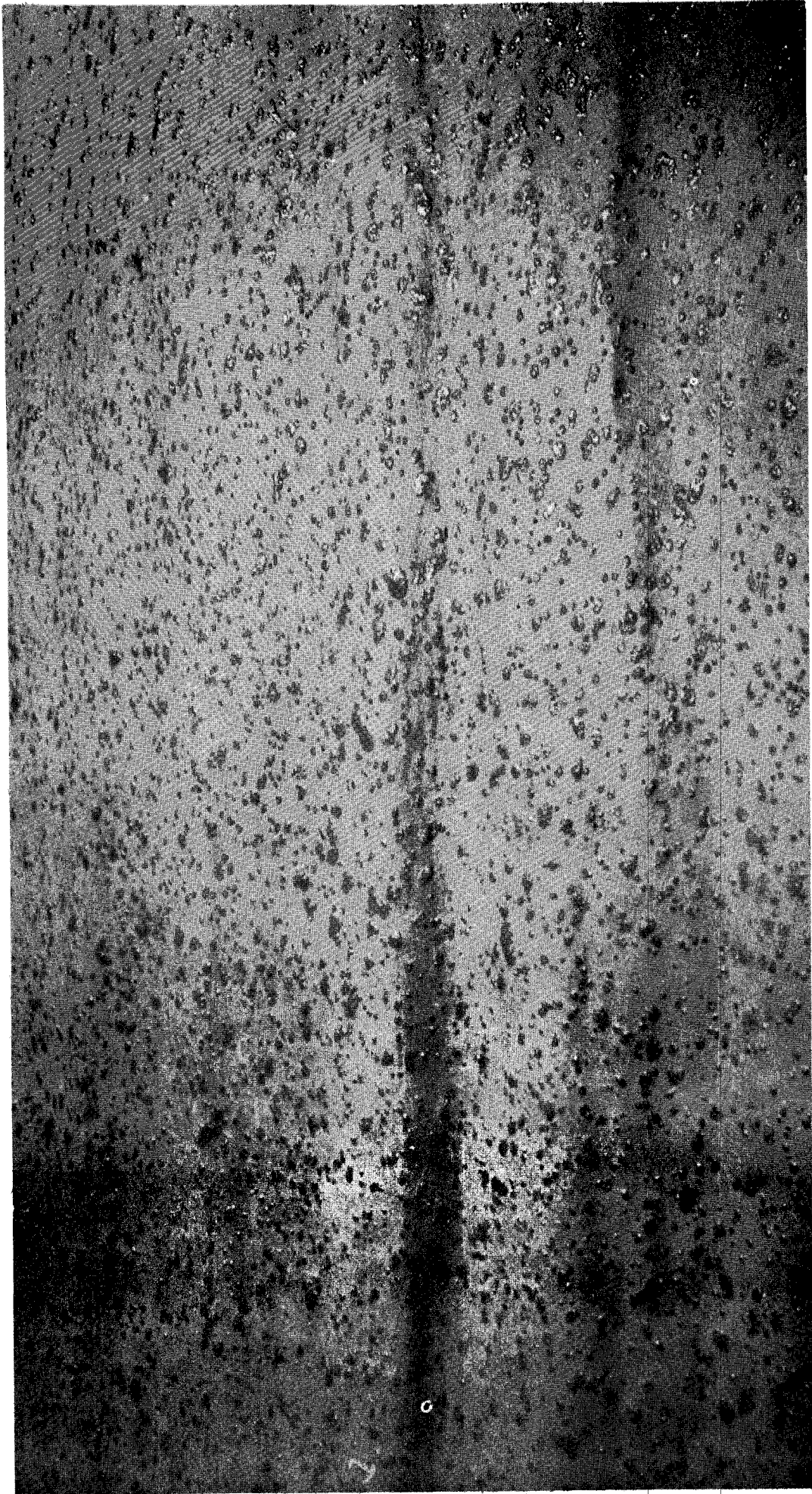
Figure 4 Spray Pattern for Suspensions
