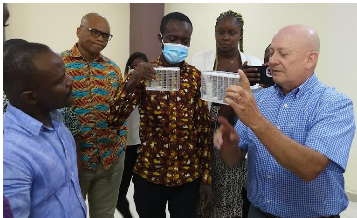
Figure 1: Demonstration of usage of the sieve box for evaluating physical properties of fertilizer products
